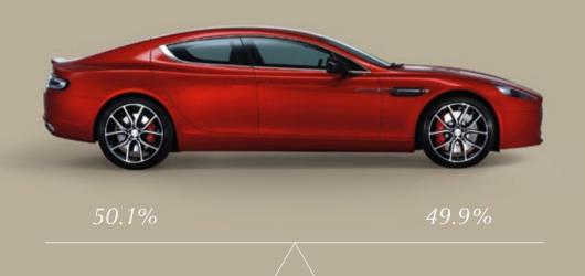
By tucking the 6.0-litre V12 engine behind the centreline of the front wheels and mounting the six-speed Touchtronic 2 transaxle at the rear, not only are the Rapide S major masses concentrated within the
